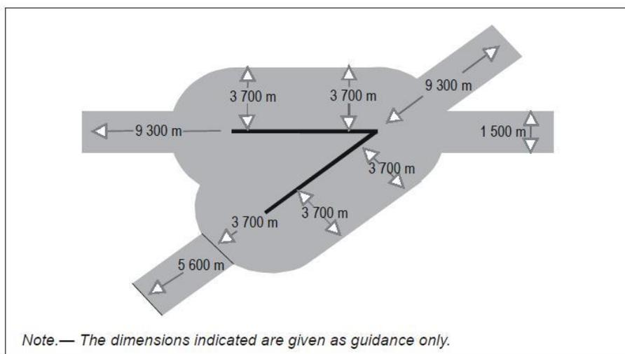
**Figure 2. Multiple runway laser-beam free flight zone**
